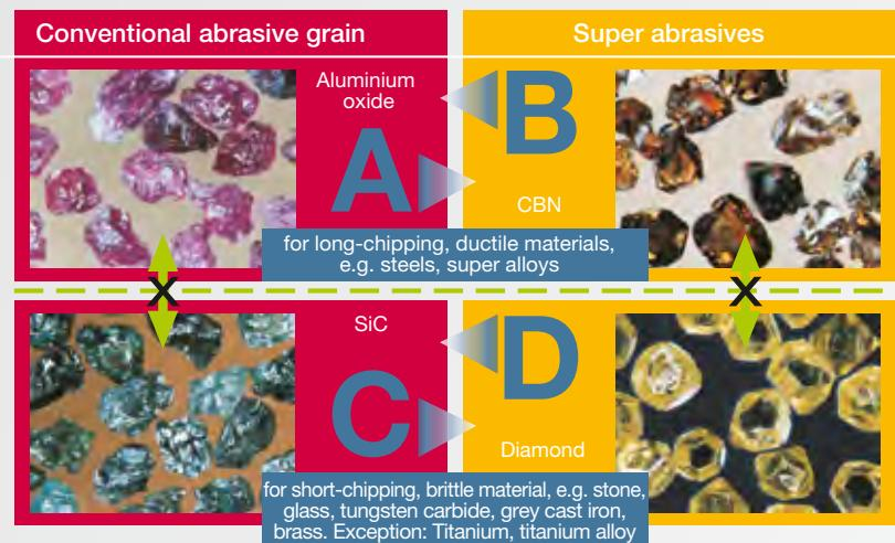
Hardness comparison of abrasives and materials. The following generally applies: The greater the hardness difference between the abrasive grain and the ground workpiece, the higher the grinding power.
